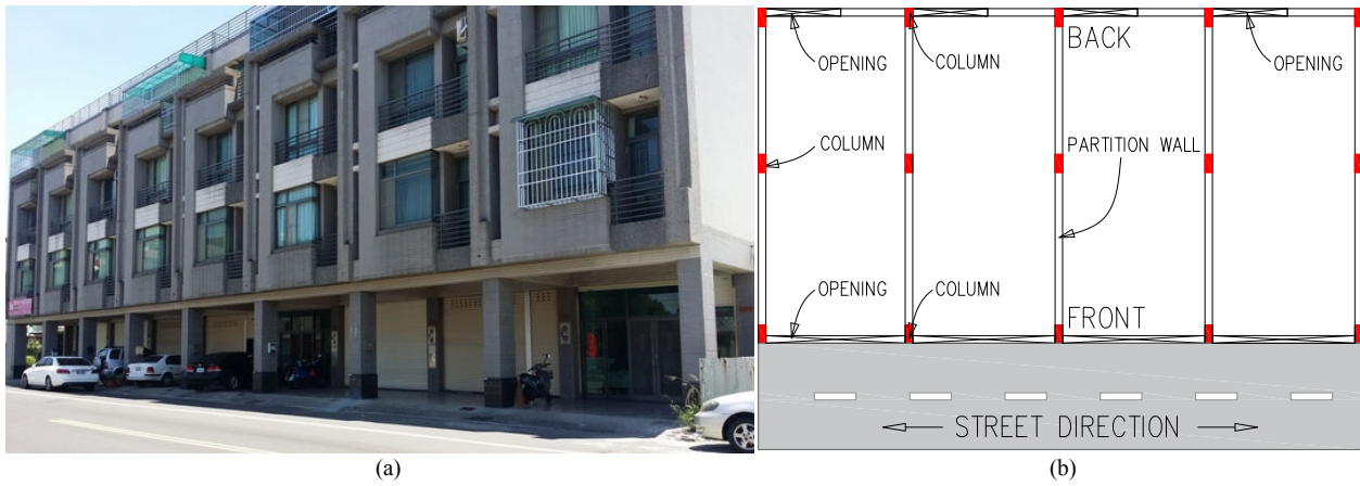
Fig. 1. (a) Typical row houses in Taiwan; and (b) plan view of the first story of typical row houses
